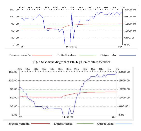
Fig. 4 Schematic diagram of PID low temperature feedback
